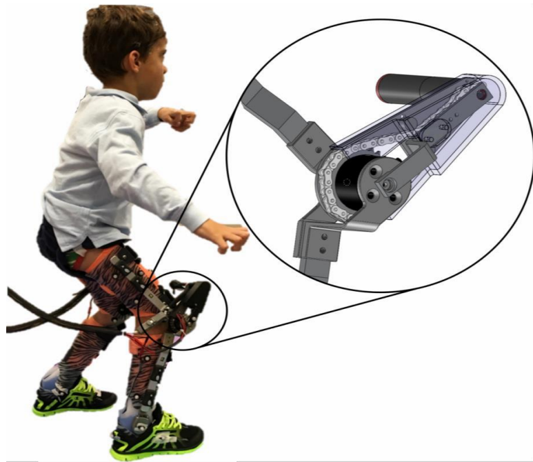
Figure 1 Adjustable Human-Exoskeleton Mounting Interface
